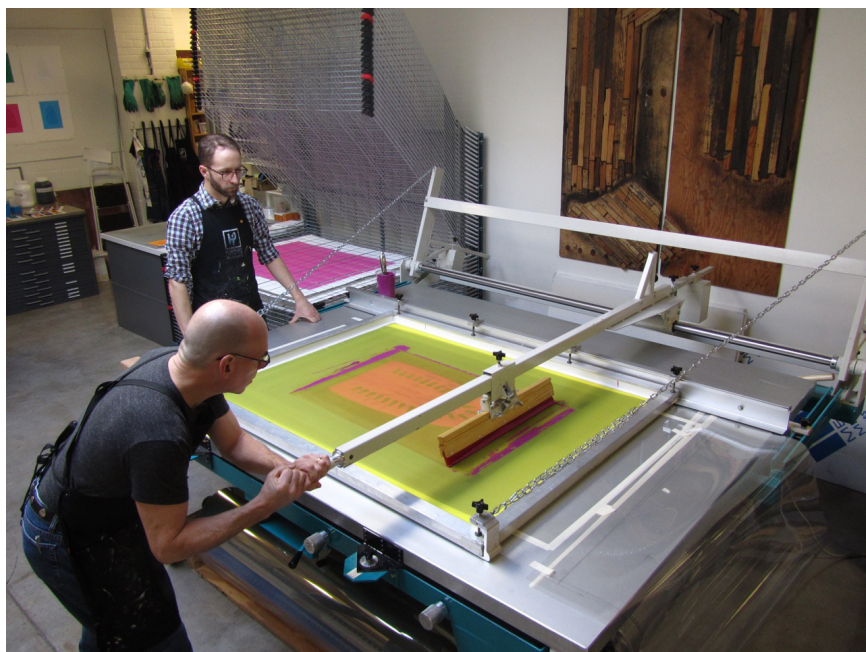
Cole Rogers, Artistic Director & Master Printer at Highpoint Center for Printmaking in Minneapolis, and Senior Printer Zac Adams-Bliss, using a large one-arm screen printing vacuum table.
